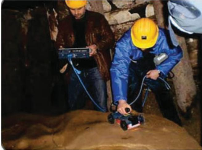
Geo-radar screening located an object inside the megalith K-2 exactly in the middle. It seems that the builders first made a base, then placed an object inside and finally closed it with the cover.
