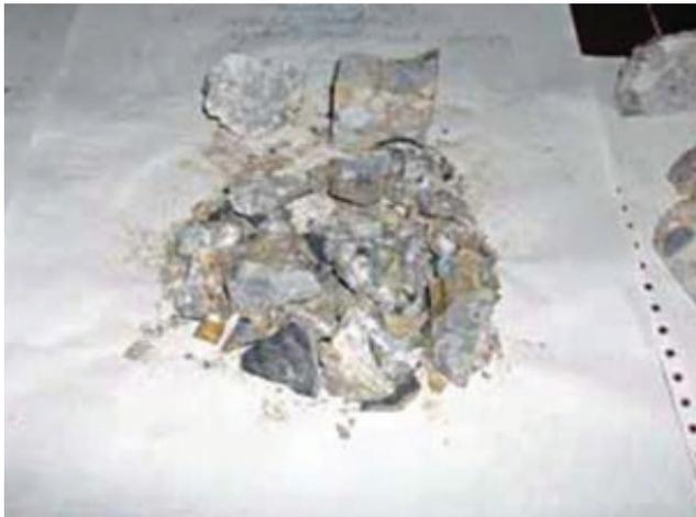
Layout of crushed test cubes of building material of covering layer at Bosnian Pyramid of the Sun, after the compressive strength test
