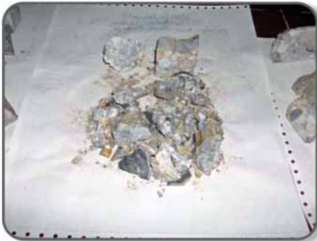
Layout of crushed test cubes of building material of covering layer at Bosnian Pyramid of the Sun, after the compressive strength test
