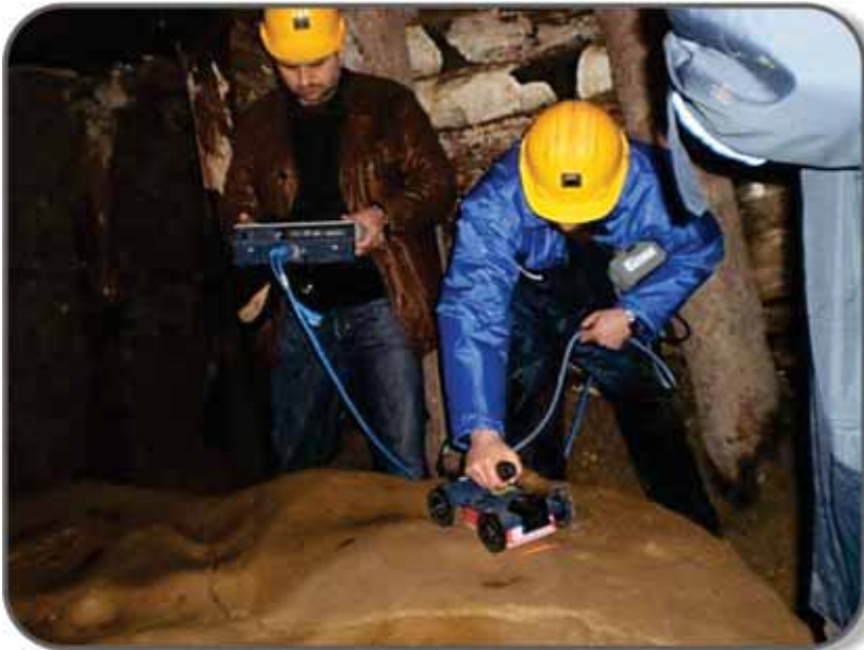
Geo-radar screening located an object inside the megalith K-2 exactly in the middle. It seems that builders first made a base, then placed an object inside and finally closed it with the cover.
