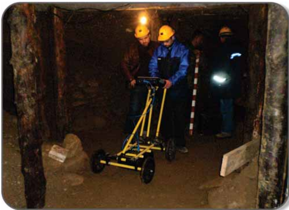
Georadar recording of underground labyrinth, "Ravne"
