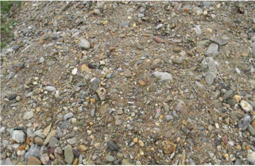
Photo 16; Image shows disaggregated Ravne conglomerate (Clasts with coarse calcareous sand matrix). This material was used to block the passages within the Ravne Tunnels complex.
