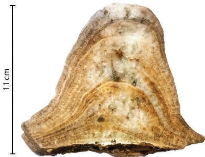
Photo 35; Stalagmite S002 was cut in half to prepare a small carbonate sample from its base for U-Th dating.
